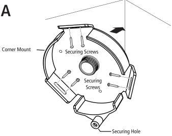
Locate the corner mount in the required position. Use screws and wall plugs (as appropriate to the wall surfaces) to fix the corner mount on the wall. Access to the screw positions is gained through the open front aperture of the corner mount.
